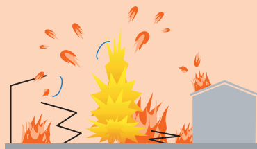
Light sheet constructions offer almost no resistance to explosions. Blast waves and burning material can spread unhindered.
