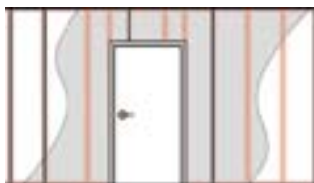
Forming door openings – front view
