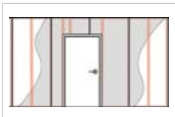
Forming door openings – front view
