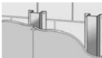
Fixing method for metal firrings
