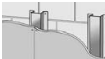
Fixing method for metal firrings
